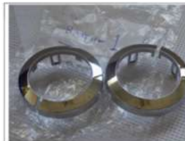
Image ID: 1/ D1704-51828 Batch - 01 Comment: Components before subjecting to salt spray .
