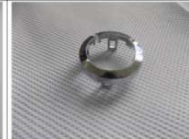
Image ID: 4/ D1705-53157 02 Comment: Corrosion observed at 72 Hrs .
